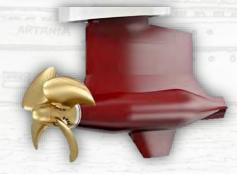
Podded propulsion or Conventional electric propulsion
