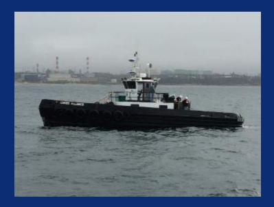
Foss Tug Boat: Brynn Foss Length = 100 feet Horsepower = 4,700 Bollard Pull = 55 tons Foss Line Boat: Caribe Alliance Length = 64 feet Horsepower 850
